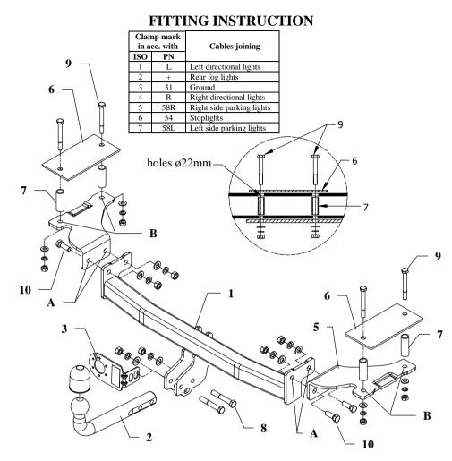
This towing hitch is designed to assembly in following car: **OPEL COMBO**, **B**, **delivery truck**, produced since 09.1995 till 08.2001, catalogue number **E20** and is prepared to tow trailers max total weight **1200 kg** and max vertical load **50 kg**.
